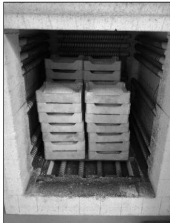
**Figure 2.** Natural dolomite calcination inside in a high-temperature electric furnace
