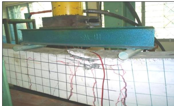
**Figure 11.** Normal beam failure under two points loads
