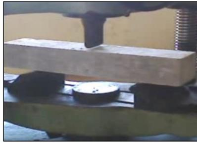
**Figure 9.** Flexural tensile strength test in Universal Testing Machine
