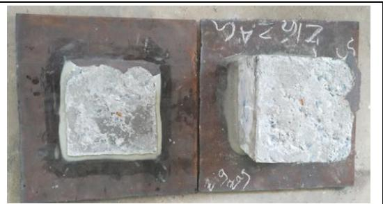
Figure 21. A typical Set 2 specimen after failure
