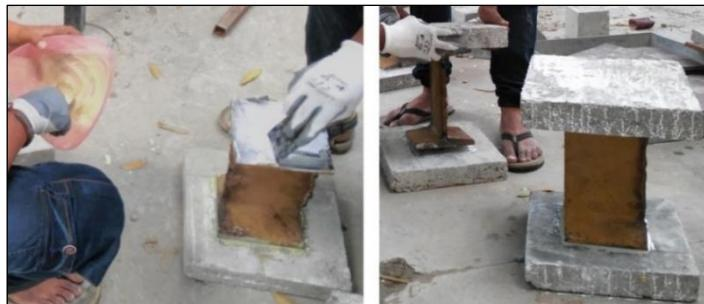
**Figure 13.** Mixing and Application of Epoxy to I-section
