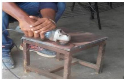
**Figure 11.** Cleaning surface of steel plate
