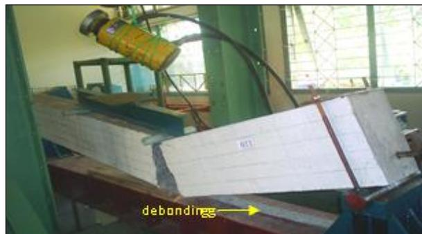
Figure 13. Beam with CFRP failed through debonding mechanism
