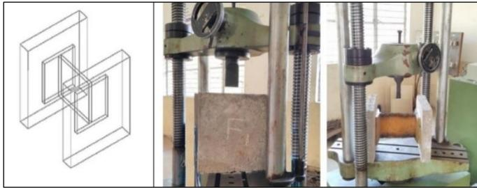
Figure 14. Arrangement of specimen in UTM and application of load on the specimen
