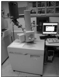
**Figure 7.** Scanning electron microscopy apparatus (JOEL model JSM-6390LV)
