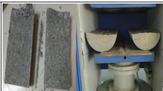
**Figure 8(b).** Test for split tensile strength
